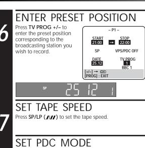
Press **PDC** to select "ON" or "OFF". If "VPS/PDC ON" is displayed on the screen or "VPS/ PDC" is lit on the display panel, PDC is set to ON. If "VPS/PDC OFF" is displayed on the screen or "VPS/ PDC" is not lit on the display panel, PDC is set to OFF. If "PDC Recording" in the right column.
